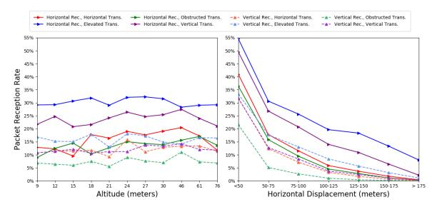
**Figure 9.** Predicted mean PRR from ZINB model for each receiver/transmitter configuration. Left: grouped by altitude; Right: grouped by horizontal displacement.
