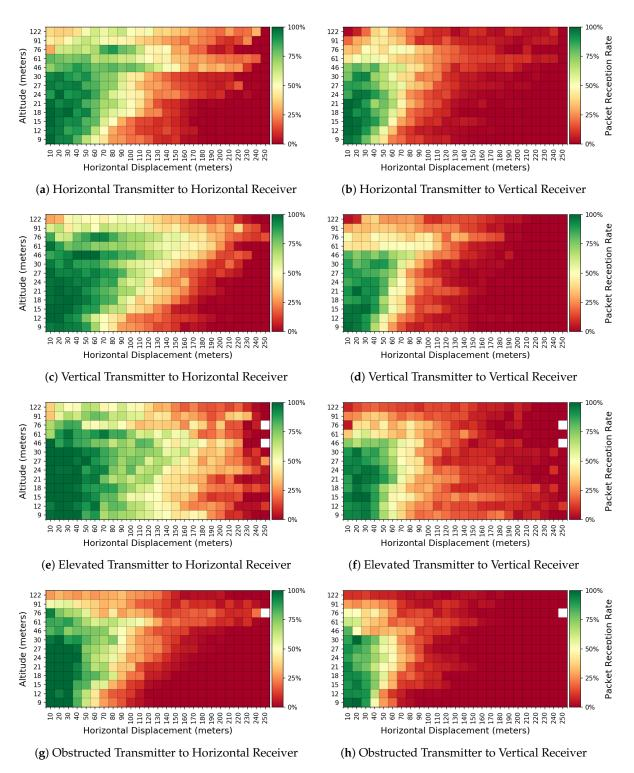
**Figure 7.** Observed packet reception rates grouped by altitude and 10 m displacements from transmitter. Cells with fewer than five sent packets are left blank.
