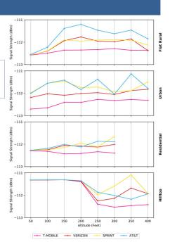
Figure 5. Signal strength change by altitude and network.
